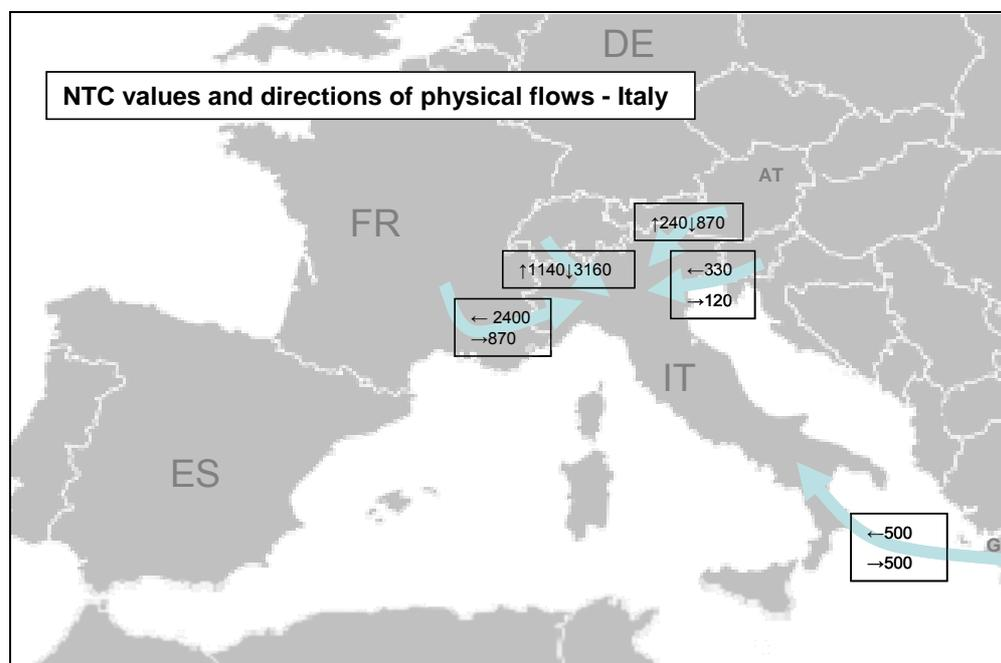
The Italian transmission grid is interconnected to the rest of UCTE Power System by means of 18 interconnection lines: four with France, nine with Switzerland, one with Austria, two with Slovenia, one underwater direct current cable with Greece and one underwater direct current cable between Sardinia and Corsica. The cross border interconnectors can be summarised in three independent axes:
