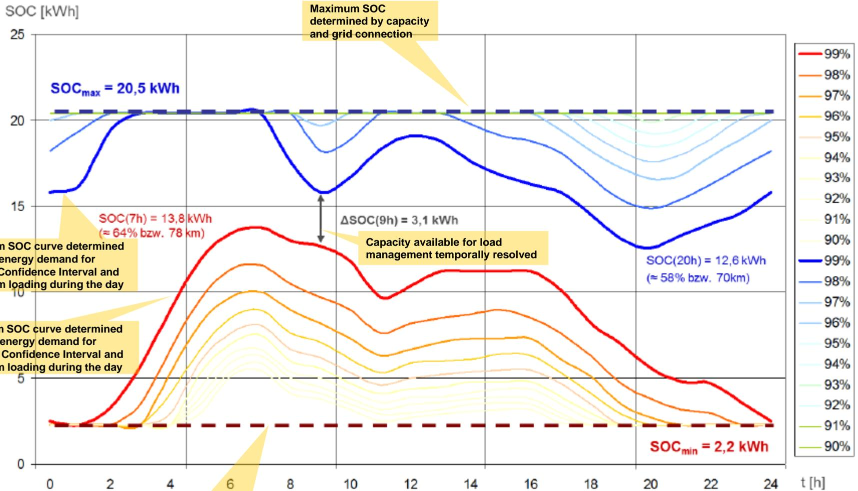
Maximum SOC curve determined by daily energy demand for driving, Confidence Interval and maximum loading during the day
